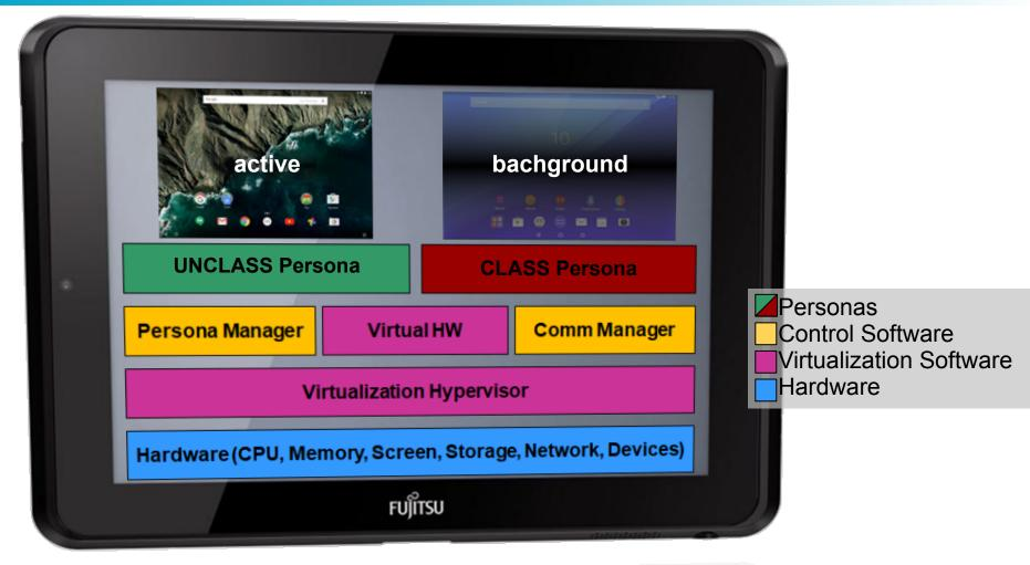
Modular system allows Freeboard to incorporate advances in virtualization, security, HW and persona SW
